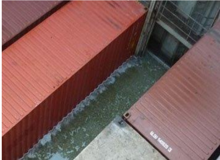
Image 22 - Container ship hold flooded – Source: UK P&I Club
