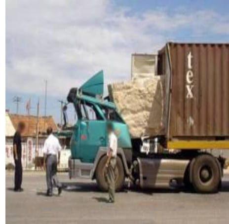
Image 28 – Granite block bursting out through the doors of a container
